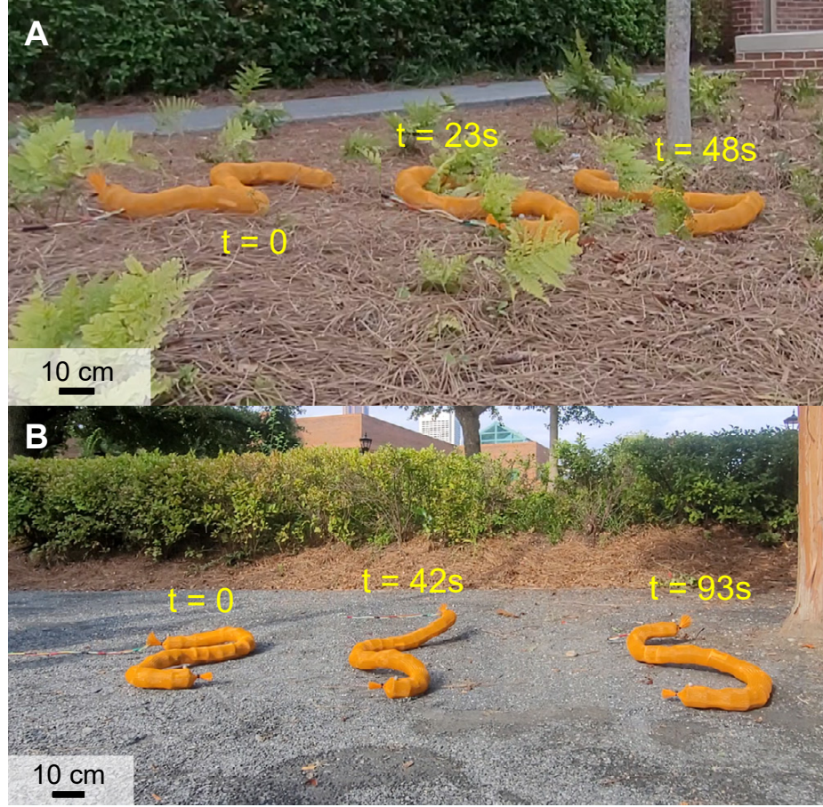
Figure 4.5: The robot demonstrates its capability of sidewinding in complex natural environments with bidirectional compliance ( G = 1 ). (A) Time-lapsed images of the robot traversing pine straw and fern environment. (B) Time-lapsed images of the robot traversing coarse granular media environment. Figures are adapted from [100].
